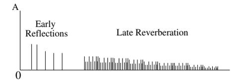
Early reflections can be calculated by considering them as sources in 'virtual rooms' surrounding the listening room (see Figure 2). Evaluating the distance and direction of these virtual sources from successive shells results in an accurate simulation of the early signal.
